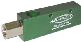
**RAV** - Large size with higher vacuum flow capacity to 14 scfm and vacuum levels to 27”Hg.
